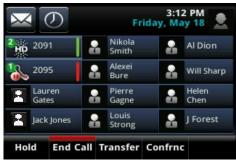
A green bar indicates a line with an active call. A flashing red bar indicates a line with one or more held calls.
