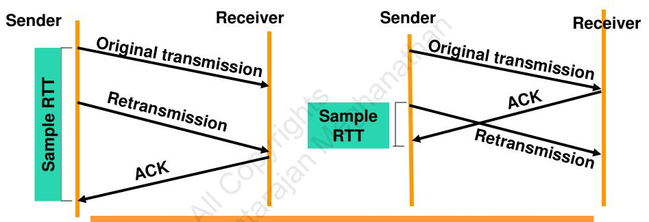
Which Sample RTT to be used to calculate the Estimated RTT? Solution: Karn/ Partridge Algorithm
