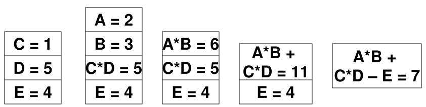
Note: During a scan of a pre-fix expression, the right operand of an operator goes first into the stack followed by the left operand. Hence, during a pop, the left operand comes first out of the stack, followed by the right operand
