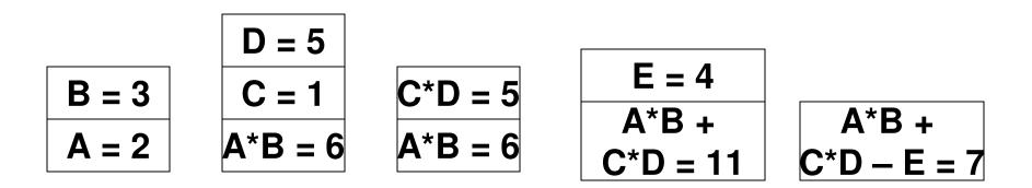
Note: During a scan of a post-fix expression, the left operand of an operator goes first into the stack followed by the right operand. Hence, during a pop, the right operand comes first out of the stack, followed by the left operand
