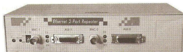
Figure 14: An Ethernet repeater with AUI connectors for 10Base5 and BNC connectors for 10Base2
