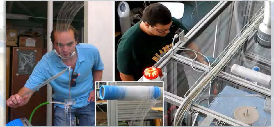
IRES PIs tests a prototype ac-electrospinning device (left); IRES scientist works with a new nanofiber yarn-making machine (right)
