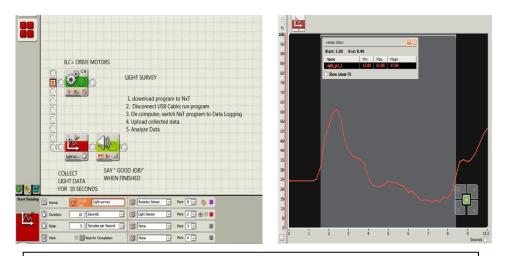
Figure 5: The NXT Robo programming for datalogging and the sensor light interruptions display
