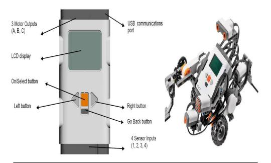
Figure 2: Lego NXT Intelligent Brick outlay and the NXT Robo with sensors and servo motors
