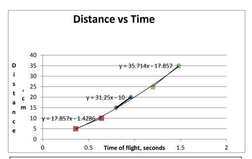
Figure 6. A plot of distance travelled by the robo vehicle (in units of cm) vs duration of the time for the corresponding distance (in units of seconds) for a NXT Robo cart on an incline.
