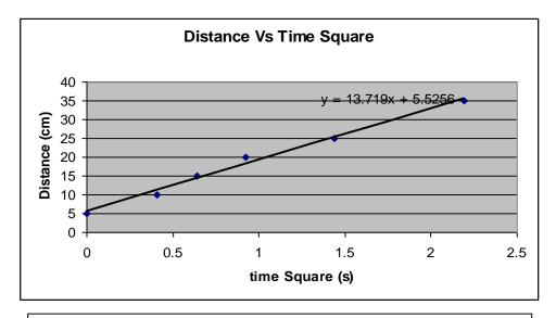
Figure 7. A plot of distance vs time squared for a NXT Robo cart on an incline
